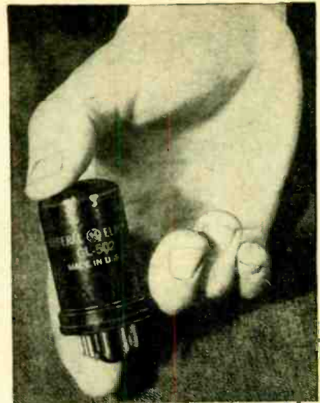
One of the smallest industrial rectifiers. Some larger ones are several feet in diameter.
